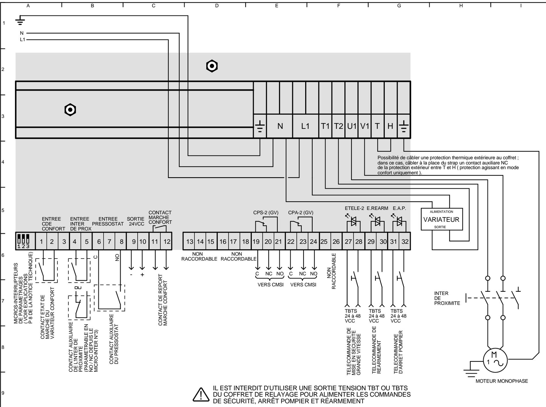
**!** IL EST INTERDIT D'UTILISER UNE SORTIE TENSION TBT OU TBTS DU COFFRET DE RELAYAGE POUR ALIMENTER LES COMMANDES DE SÉCURITÉ, ARRÊT POMPIER ET RÉARMEMENT
